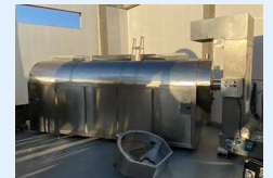
烘炒設備 Roasting Equipment
